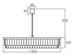
The dimensions of the central supporting rod and ceiling rose are not included in the height measurements. The standard rod and ceiling rose is 50cm (20") high if not otherwise specified by the customer.
